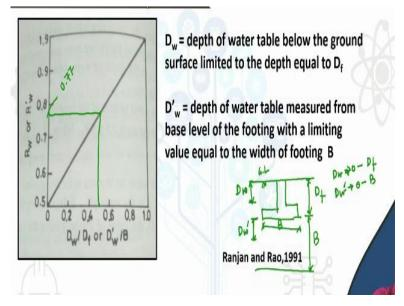
The two water table correction factors ( $R_w$  and  $R_w$ ') depend upon two depth values  $D_w$  and  $D_w$ ' defined as:  $D_w$ - depth of water table below ground surface, limited to  $D_f$  and  $D_w$ '- depth of water table measured from footing base limited to B. So,  $D_w$  varies from 0 to  $D_f$  and  $D_w$ ' from 0 to B. The values of  $R_w$  and  $R_w$ ' can be obtained by calculating  $D_w/D_f$  and  $D_w'/B$  respectively using the graph shown in the slide above.
