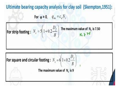
The next bearing capacity equation I will discuss is the Skempton bearing capacity equation, proposed by Skempton in 1951 which is applicable only for clay. Terzaghi's bearing capacity equation is applicable for  $c-\phi$  soil, clay, sand and also the mixed  $c-\phi$  soil, but this bearing capacity equation is applicable for clay. Generally, I would recommend this equation to design a foundation on clay.
