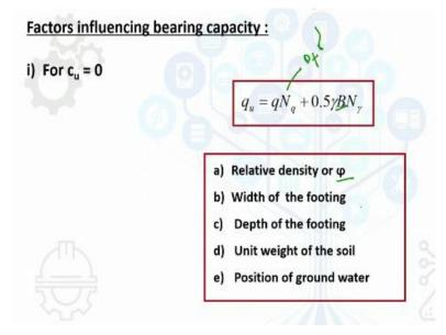
Now, let us look into the factors influencing bearing capacity. If the footing rest in a soil for which c = 0 (cohesionless soil), the first term in the bearing capacity equation,  $cN_c$  will be 0. So, the equation will be  $qN_q + 1/2$  ( $\gamma B N_{\gamma}$ ). So, the factors affecting this equation would be:  $\phi$ , width of footing (B), unit weight of soil ( $\gamma$ ), depth of footing (D<sub>f</sub>) [Since,  $q = \gamma D_f$ ] and the position of water table.
