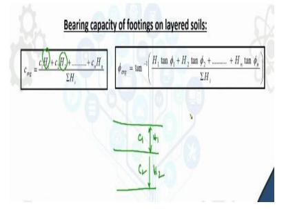
The equations mentioned so far can be easily applied for homogeneous soil. But if the soil is layered, these equations cannot be directly used. In general, the weighted average of cohesion and friction values will be calculated.  $c_1$  is the cohesion of the first layer,  $H_1$  is the thickness of the first layer;  $c_2$  is the cohesion of the second layer and  $H_2$  is the thickness of the second layer.
