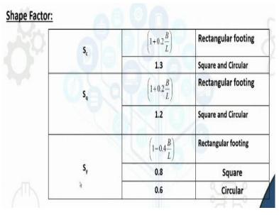
IS code also gave the shape factors  $(S_c, S_q, S_\gamma)$  for rectangular, square and circular footings. (Refer Slide Time: 21:32)
