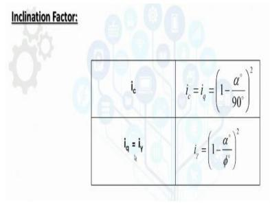
The inclination factors  $i_c$ ,  $i_q$ ,  $i_\gamma$  are also given in terms of  $\alpha$  where  $\alpha$  is the angle the inclined load makes with the vertical.
