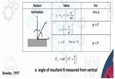
Similarly the inclination factor expressions are also given where,  $\alpha$  is the angle the load makes with the vertical. With the help of these equations, we can determine these inclination factors for different  $\phi$ . The K<sub>p</sub> used in these expressions is nothing but:
