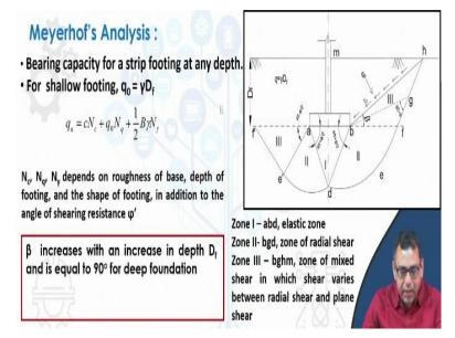
The third bearing capacity theory in our discussion is the Meyerhof's analysis okay. So, Meyerhof's analysis can be applied for. The Terzaghi's bearing capacity was initially applicable for strip footing but later on modified for circular, square and rectangular footing.
