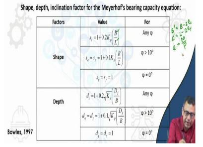
When the load is eccentric, the full width of the footing cannot be considered, as the effective width or length which actually bears the load will be lesser than the original footing
