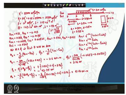
This was the problem for which the deflections at point A, B and D were calculated. Let us determine the deflection at C point first. The deflection at point D is -0.11 mm, deflection at point A is 7.83 mm and the deflection at point B is 7.53 mm. When considering deflection at point C, it is the centre point of load and so the distance from A to C and B to C is equal to 1/2. (**Refer Slide Time: 01:40**)
