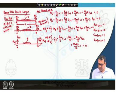
Till now the infinite beam and semi infinite beam have been discussed. The next concept is the analysis of beam with finite length. In case of infinite beam, the beam was infinite on both the sides from the loading point (right side & left side) and in a semi infinite beam, only one side was infinite and the other side was finite. But in beam with finite length both the sides of the beam will be finite and it means that the length of the beam is now finite.
