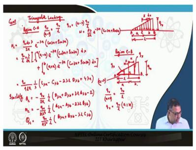
The four equations for deflection, slope, bending movement and shear force when an infinite beam is subjected to triangular loading were already discussed.
