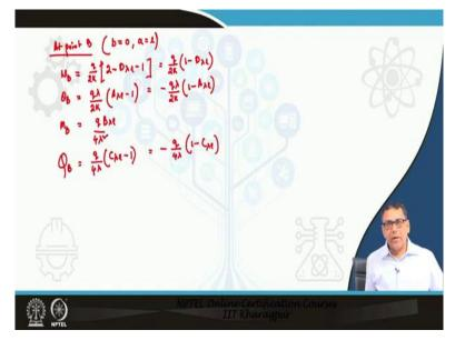
The above slide shows the equations for deflection, slope, bending moment and shear force at point B.
