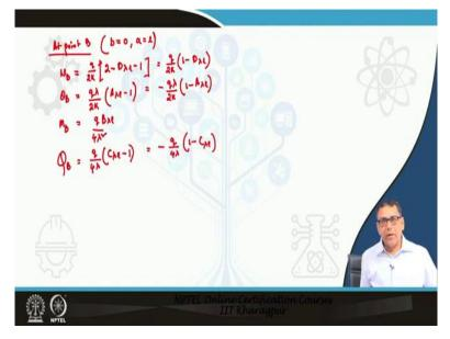
When the point of interest is B, b will be equal to 0 and a will be equal to 1 because here, point C and point B are same. Substituting these values in the equations of deflection, slope, bending moment and shear force, we get:
