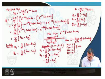
Similarly the expressions for slope, bending moment and shear force can be determined. The general expression for slope under point load is:
