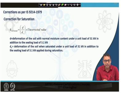
Then next correction, as suggested by the IS code is the correction for saturation. The equation for this correction is shown above where d is the deformation of the soil under normal moisture condition when a unit load of 31 kN in addition to the 3.1 kN is applied (a total load of 3.1 kN + 31 kN),  $d_s$  is the deformation of the soil under saturated condition when a unit load of 31 kN in addition to the 3.1 kN is applied.
