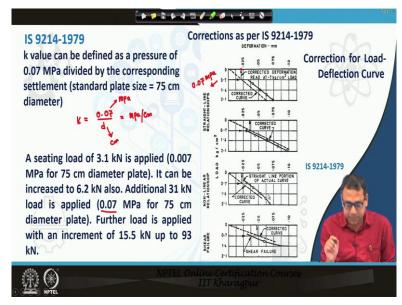
Let us have a brief overview of the method suggested by IS code 2914 1979 to determine subgrade modulus of a soil. The formulation, according to IS 9214-1979 for subgrade modulus is that k is equal to 0.07 (MPa) divided by the corresponding settlement. The plate load test should start only after the application of a seating load of 3.1 kN followed by a load increment of 31 kN which is equivalent to 0.07 MPa for a 75 cm diameter plate.
