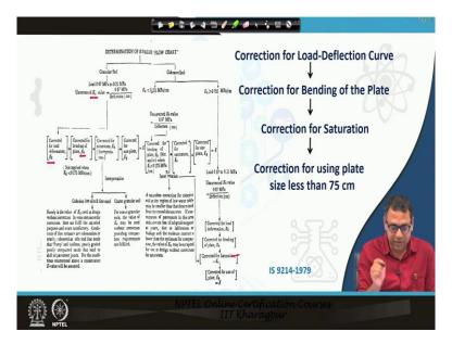
This is the summary of all the corrections discussed so far. For an uncorrected k value, the first correction to be applied is the correction for load-deflection curve followed by the bending of plate correction, and the correction of state of saturation and finally the correction for plate size if plate size used is less than 75 cm.
