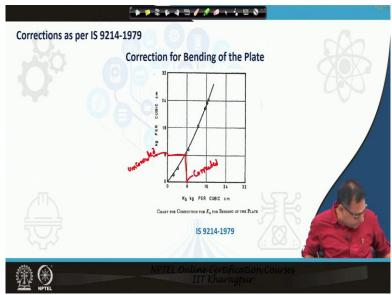
The next correction to be applied is for the bending of plate which can be determined from the graph with uncorrected k value on the Y-axis and the corrected k value ( $k_b$ ) on the X-axis.
