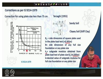
The third correction is for the plate size which need not be applied if the size of the plate is 75 cm. If the size of the plate is less than 75cm, the size correction should be applied. The IS code has recommended with this chart where this dotted line is the theoretical curve and firm line is
