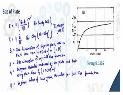
The above slide shows the equations of plate size correction in case of both sandy and clayey soils.  $B_1$  is the side dimension of square plate used in plate load test (usually = 0.305 m) and B is the dimension of any full size foundation.
