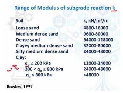
Similar to the ranges given for  $k_1$  values, depending upon the soil type, ranges for k value were also given by Bowles (1997).  $q_u$  is the unconfined compression strength of soil which was discussed in the first class ( $q_u = c_u/2$ ).
