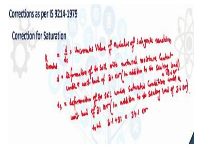
So, uncorrected value of subgrade reaction is under natural moisture content condition. In the next class, I will solve one example problem and then I will show how to determine the k value as per IS method. Thank you.
