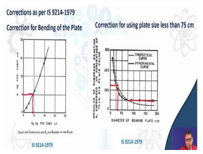
The next correction for the subgrade modulus is the correction for bending of the plate. The chart that helps to apply this correction is given in the IS code which is shown in the slide above. There are two curves given in the IS code for the bending correction. If the plate load
