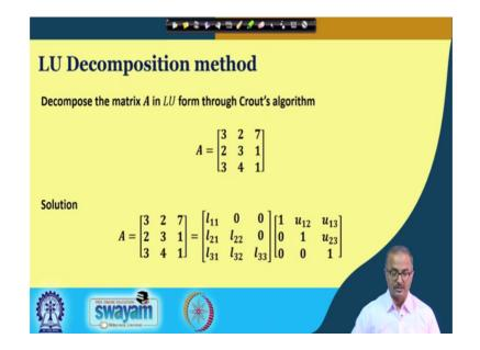
Now, we take this example problem. So, this is the A matrix given to us and this is how we are going to now find out that how we are going to decompose this A matrix in a l and u matrices with the Crout's method.
