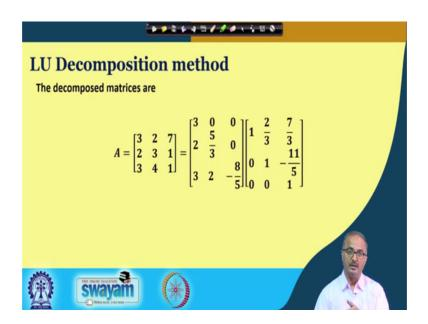
So, here you have the lower triangular matrix and the upper triangular matrix ok. So, here we have the basic thing is this we have learned how to decompose a matrix into 1 and u matrixes.
