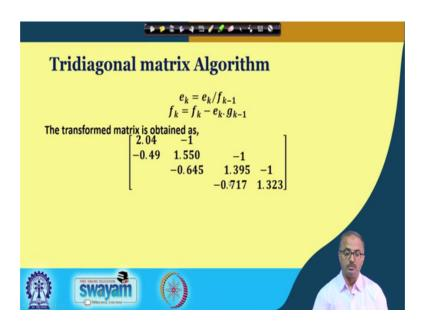
And here we have demonstrated with a example problem that how you can get the LU Decomposition method to obtain the to a solution for a Tridiagonal matrix system.
