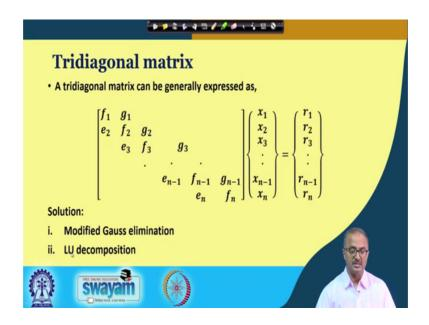
So, here as I have shown you that this is the tridiagonal matrix system. Here you have the main diagonal, this is the super diagonal, and this is the sub diagonal elements and here we have all the unknowns to be solved for and here we have the or the forcing functions. Now these can be done this can be solved by two ways, one is that we can modify that Gauss Elimination method and another is the we can use the LU Decomposition method.
