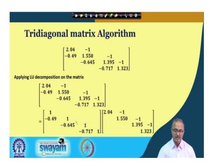
So, here you can see that as you apply the LU Decomposition algorithm you find that at each step you are able to get that how the values are getting modified and ultimately you are getting these two matrices in this is the l matrix and this is the u matrix ok.
