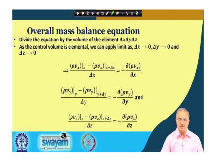
So, that is what we are doing that because, they are very small you are finding that these all this difference equations are leading to differential equation ok. So, we are writing all the differential equation like this for the three directions.
