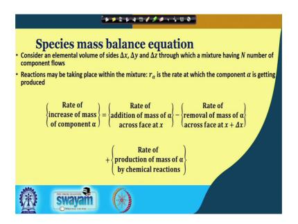
Now, let us go to the species mass balance equation. In this case as we have done previously again we are doing the mass balance over the same control volume with these delta x delta y delta z at the width in the three direction for the control volume. And, here we are considering that there is some kind of reaction going on with respect to a species alpha.
