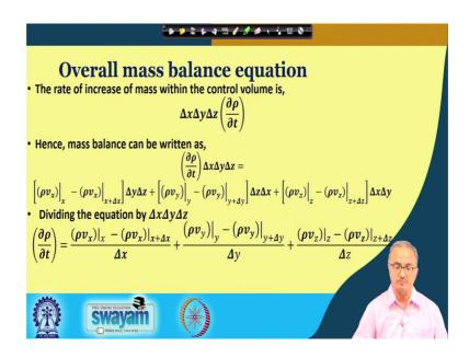
Now, you see that at what rate the mass is changing within the control volume. So, again what we are doing? We are doing that how the density is changing that is dou rho by dou t row into the volume is the mass change ok. Now, because these particular delta x delta by delta z are remaining constant; so, we are taking it out of the differential. So, we are left with that density with the differential with respect to time.
