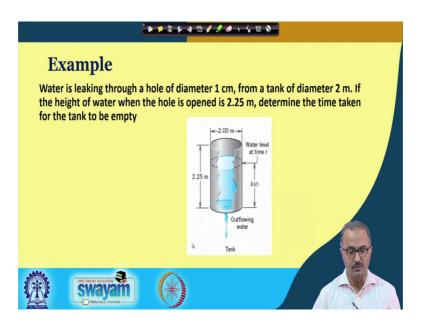
Now, we come to another the application of those form that those that method for a practical problem. What we have given is this; here we have a water tank which is leaking here ok. So, the water is leaking through a hole of diameter 1 centimeter. So, there is a hole at the bottom of the tank and water is flowing out of this hole. And this kind of system happens many at times.
