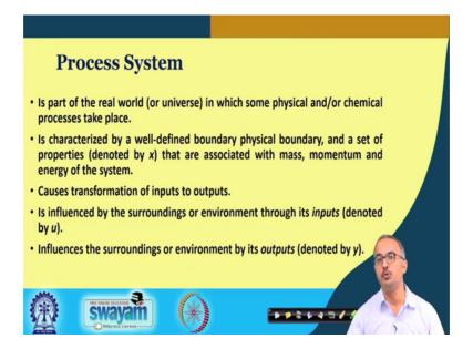
Now, you see that first whenever we talk of balances first you to identify, the system which we need to study or for which we need to make the balances and always we can identify the system properly, we cannot write the balanced equations. So, what first you to understand what we mean by a system; a system is a part of the real world or what we call the universe in which some physical or chemical processes take place.
