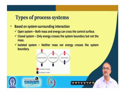
Now, we come to another basis of classification and that is based on the how the system is interacting with its surroundings. So, in the first we have the open system open means whenever we talk of these interactions, we talk in terms of the mass and energy ok. So, when we talk of open system it means that across the system boundary both mass and energy can flow either from the system to the surroundings or from surroundings to the systems so is in this is an open your system.
