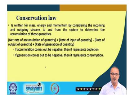
Now, once we learnt about the different systems and the properties and degrees of freedom, now we are ready to look into the balanced equation. And in this case, we go with the conservation law. And the conservation law is about that net rate of accumulation of a quantity within a system is equal to the rate of input of the quantity minus rate of output of the quantity plus rate of the generation of the quantity ok.
