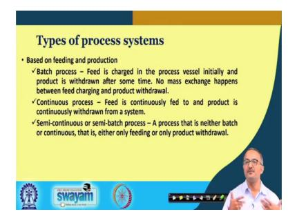
Another classification is based on the feeding and the production of the in the particular system. Now, feeding and production you can see from this example that we have batch
