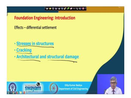
Similarly effects of the differential. What are the different effects of differential settlement? As I told you the differential settlement is the harmful the stress in the structure. So, if the if the building is there, if it is settled like that, if it settled this side, then automatically these will be extra stress on the building elements like beam, column or wall, and then automatically there can be cracks, and there can be architectural and structural damage.
