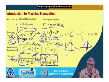
So, now, let me go to and I have told you that 2 solution I have shown for constant force system and rotating mass system. And you can see that the solution important thing you have to remember that when the force is F naught sin omega t and when force equal to m e e omega square sin omega t. In that case resonant frequency will be over will have omega n over resonant will occur at omega will be equal to these or omega over omega n will be equal to 1 under root 1 minus D square.
