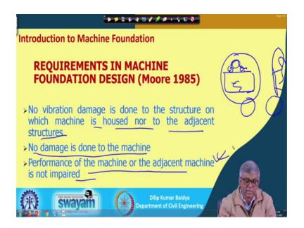
Now, let me quickly go to the requirement for foundation design for vibrating load. So, no vibration is done to the structure on which machine is housed; that means, if I put a machine over this foundation this foundation should not be the damaged or to the adjacent structure also. So, because of the vibration of that the adjacent structure should not also be damaged.
