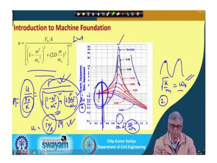
So, that is a solution actually general solution you can see that u actually displacement amplitude of course, sin omega t can be there here, but this is the maximum temperature at a particular frequency this is the maximum amplitude. So, displacement maximum; that means, if you have this then this is the one by these expression it is giving that one ok.
