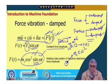
And in this you can see that, we have discussed 4 different types of vibration analysis that is free vibration and force vibration under that it is undamped and this is damped and here also similarly undamped and damped ok.
