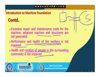
Next one I can see that excessive repair and maintenance. So, if I do not designed properly then you may require excessive maintenance or repair cost that has to be prevented. Performance and health of the worker is not impaired; that means, what if you allow too much of vibration in the system then during vibration, what will happen that people working in the around surrounding places. They may not be that environment, may not be comfortable or it may be a health hazard may occur.
