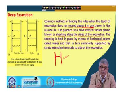
So, this one is shown here actually there are different types of supporting systems are possible; actually when the comparatively shallow excavation suppose 3 to 5 meters. You can see here the common methods of bracing the sides when the depth of excavation does not exist 3 to 3 meter actually, that will be done actually that there will be wooden sheets will be inserted and then there will be some support will be there like that.
