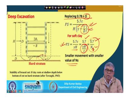
So, that this entire failure mechanism is prevented in that case you can see that 0.7 B instead of that I can restrict now D only. So, you can there actually we have shown that B bar we have replaced by 0.7 B. So, there actually instead of 0.7 B now you can put D.
