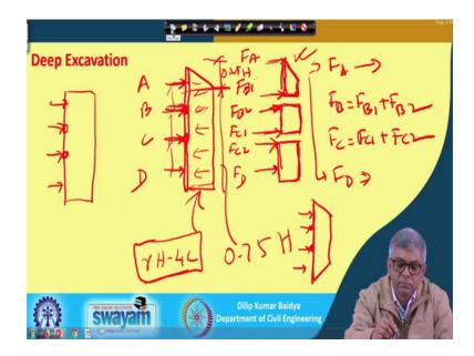
Next slide actually I kept blank and I will just show that how it will be done; let me show you this way. Suppose there is a; this is the excavation and your strut actually somewhere here, somewhere here, somewhere here like that. They are maybe uniformly spaced and suppose based on the soil type the pressure diagram something like this suppose ok. So that means, I will consider now this has a beam and these are the actually your pressure loading.
