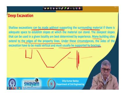
And, you can see here next slide what I tried to show here you can see that shallow excavation can be done without any support as we have shown theoretically up to some depth we can theoretically; up to some depth without any support vertical cut. Suppose, if there is a cut is this much depth and if it is based on the calculation order the; if it is this much we may be able to do without support.
