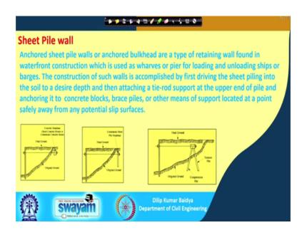
Cantilever already we have done, anchored sheet pile wall which is also known as bulkhead, anchored bulkhead are type of retaining wall, found in waterfront construction mostly, which is used as a wharves or pier for loading and unloading ship or barges and how it constructed actually. Generally this construction of this type of wall fast, it will be penetrate and desire depth.
