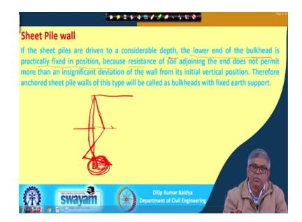
But next let me show if it is ah, what is fixed earth support? See that is the fixed earth support this is, if the sheet piles are driven to considerable depth, the lower end of the bulkhead is particularly fixed position because. So, that is what we have got something
