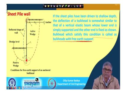
Next part is actually that anchor bulk head and if you see typically if it a, penetration is very deep and it can be deep or it can be shallow. When the penetration is shallow then your typically anchor bulkhead that deflection shape will be like this. It is shown here actually deflected shape will be like that and this portion will be keeping like almost like simple support ok.
