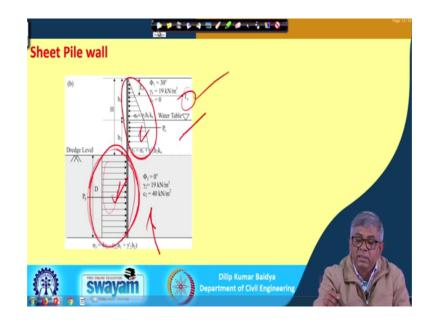
Now, I will go to next slide. So, this is the one I have told you that similar to your cantilever sheet pile wall, even bulkhead also it can be of combination of above dredge level, suppose sand, above dredge level sand and below dredge level actually your clay, then corresponding pressure diagram is like that. If this pressure diagram like this then your problem actually, again it becomes simpler, in that, I have not done this, but if you want you can do it, same way it can be done.
