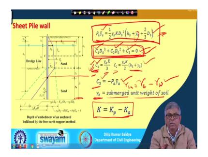
So, next one, you can see now P a y a bar, y a bar is this equal to so; that means, P a y bar equal to half gamma b K D naught square plus h 3, so this is written correctly here; h 3 y naught plus 2 y 3 D naught. And then this one if you simplify, this one if I simplify then it will reduce to equation C 1 D naught cube plus C 2 D naught square plus C 3 equal to 0.
