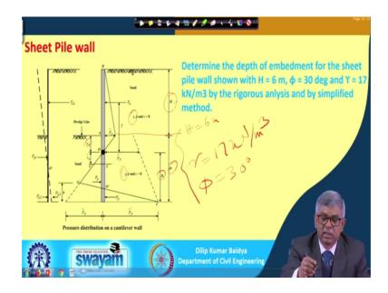
So, this is the problem actually, problem is like this determine the depth of embedment for the sheet pile wall shown with H equal to 6 metre phi equal to 30 degrees and gamma equal to 17 kilo Newton metre cube by the rigorous analysis and by simplified method. There are two method actually we have to use and that is how this is the wall actually this dredge level. So, here actually H equal to 6 metre; so, H equal to 6 metre and your gamma hare gamma here.
