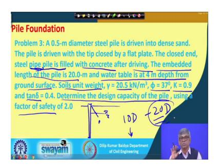
So, third problem actually you can see here the pile driven in pile driven in sandy soil. And you can see that a 0.5 m diameter steel pile is driven into dense sand. The pile is driven with the tip closed by a flat plate ok; that means, it is a hollow actually, bottom is closed initially while driving. And the closed end, steel pile is filled with that is pipe pile actually closed end the closed end steel pipe pile steel pipe pile is filled with concrete after driving.
