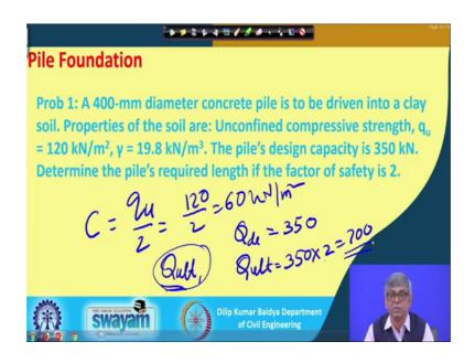
So, let me see two to three problems now. First problem is actually you can see here a 400 mm diameter concrete pile is to be driven into a clay soil. And properties of the soil are unconfined compressive strength q u is 120 k N per m square, unit weight gamma equal to 19.8 k N per m cube. And pile's design capacity is 350 k N. Determine the pile's required length if the factor of safety is 2 ok.
