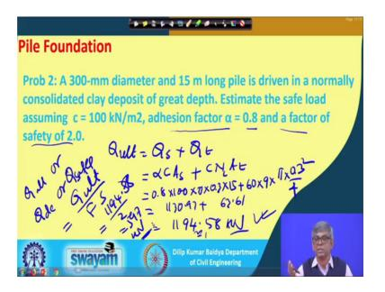
Let me go to the next problem. So, next problem also similar the pile is driven in again clay soil instead of L is unknown now I am this is giving you L and you have to find out the design capacity of the pile. You can see here that a 300 mm diameter and 15 m long pile is driven in a normally consolidated clay deposit of great depth that mean the soil up to sufficient depth beyond 15 meter also same soil, so that I can use the value of property of that layer.
