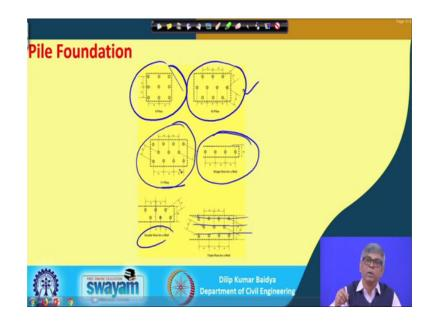
Similarly, if there are 9 piles so, this will be the best way of configuring and if it is suppose 10 pile, suppose this may be the best way of configuring and each here.
