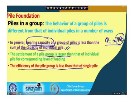
So, let me start with the first slide as I have mentioned already that the piles in a group the behavior of a group of piles is different from that of individual piles in a number of ways. That means, not only one reason or one point that it is different only this there are several ways in different. And in general you can see bearing capacity or of the group of piles is less than the sum of the capacity of the individual pile.
