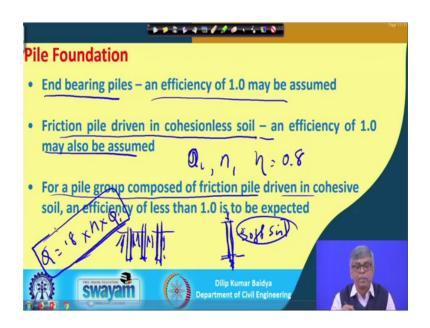
Next I can see that the as I have told that that capacity or efficiency may vary depending of spacing, then type of soil and then function of the pile, how it is transferring the load all mechanisms. So, in when pile is n bearing n bearing pile means what? This pile is here and he here and load is applied here and there may be the only bearing from here. This is so loose soil loose or topsoil suppose here. So, in that case, there is no resistance only there is a steep layer or rock layer.
