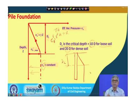
You can see now the diagram again drawn here where neatly. You can see here if I calculate sigma V dash at any point suppose here. Sigma V dash if I calculate here how what will be here it will be if it is no water table if it is no water table it will be gamma times H. And if it there is water table some it is under water table it is gamma some are time being because it is effective vertical stress you have to calculate actually effective vertical stress ok.
