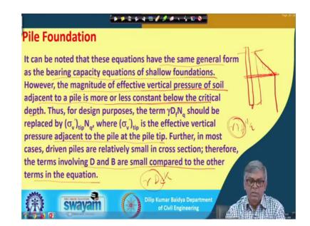
Now, you can see here some discussion I have made here. It can be noted that the equation have the same general form as the bearing capacity equation of shallow foundation as I have already mentioned. The magnitude of effective vertical pressure of soil adjacent the pile is more or less constant below the critical depth is not.
