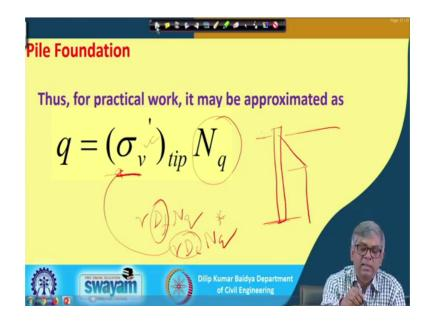
We express by this equation we consider q equal to sigma v dash tip N q. And this N q is not the same N q of shallow foundation N q. We will discuss that actually the a subsequent lecture. For the time being I will tell you that sigma v tip means if there is a pile something like that then gamma D f actually has a your equation says gamma D f N q. .
