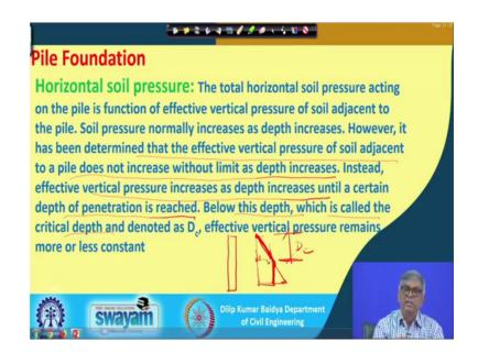
And horizontal soil pressure this is the one very important as already I have explained that way. And you can see that horizontal soil pressure this is the pile, 1 second I will do here. And at this point suppose I want to do horizontal pressure at this point vertical pressure 0 then horizontal pressure also 0. At this step horizontal vertical pressure will be some value horizontal pressure also bigger than 0.
