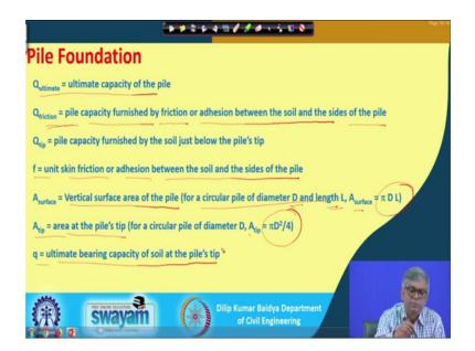
And you can see I have again elaborately defined all those term Q ultimate means; ultimate capacity of the pile Q friction means pile capacity furnished by friction or adhesion between the soil and pile and the sides of the pile. So, Q friction so Q f or sometime Q s is nothing, but pile capacity furnished by friction or adhesion between the soil and the sides of the pile.
