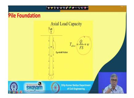
So, we will just continue with that let me. So, I have shown actually earlier that pile actually axial pile, but it is for compression. And we have seen that there was a tip resistance and there was a frictional resistance frictional resistance and tip resistance. But pile can be also used as a uplift actually tension in that case you can see here if that T ultimate applied here.
