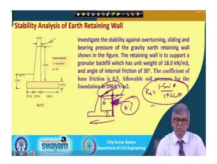
So, this wall suppose this is the wall here and this is the wall. So, this inclination is there. Instead of that instead of that, I may give I may we may express horizontal in that case your wall height will be only this much. You extend from here and this will be wall height. So, this will be wall height will not change here or wall height will change only when there is a level backfill ok. So, here wall height would be it was 6 and it was 0.7. So, it be wall will be 6.7.
