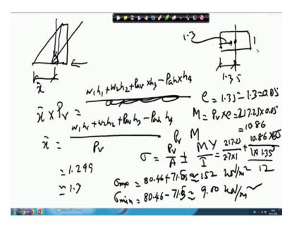
Suppose, this is the base of the this is this is the one and different forces are acting at different point. So, I can find out that vertical pressure resultant vertical pressure acting somewhere somewhere here and then or in some angle actually acting pressure are maybe some angle and then I can consider vertical and horizontal and suppose these distance is suppose x bar.
