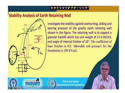
You can see here this wall actually is actually 5 meter high and you can see there is a gravity retaining wall and this back side is vertical and it has a 2.7 meter width at the base and this wall is perpendicular to the board here I can consider a infinitely long that can be long enough which I consider as long enough and for that I can analyze for a unit length. So, that means, I can take this base I can consider as 2.7 this is 2.7 and I can take unit width of 1 meter.
