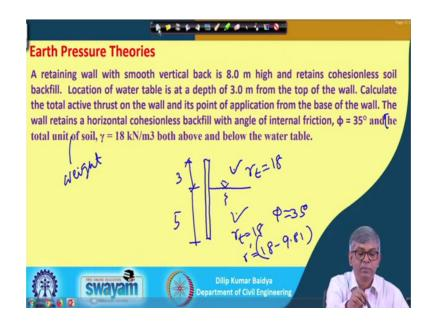
You can see that retaining wall with smooth vertical back 8 meter high and retains cohesion less soil backfill. Location of water table is at a depth of 3 meter from the top of the wall. Calculate the total active thrust on the wall and its point of application from the base of the wall. The wall retains a horizontal cohesion less backfill with the angle of
