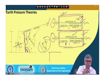
Now, there is a Coulomb's theory. In it in this actually this is very much universal that means, the some of the assumption can be eliminated that means, actually we can see this is as per Coulomb's theory that it can be any angle this instead of back vertical wall. It can also inclined backfill, back also in inclined sorry, wall back also can be inclined you can see this is very common also in many cases.
