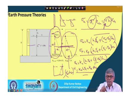
For example, so this is the wall and this is the wall and water table is here though it is same soil granular soil, but water table was here. Now, previously it was dry, but here it is water table is there. So that means, I can find out K a K p at the same way it will not change it will not depend on earth pressure water table condition, it depends on the soil type only, but your earth pressure diagram will change total thrust also it will change because of this water table location.
