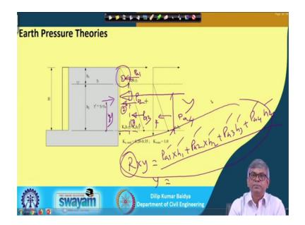
So, if this is the diagram actually, if this is the diagram we can see I can divide into this is part 1, I can divide in to part 2, I can this is 3 and this is 4. Now, I can consider at this one as P a 1, I can consider these as P a 2, I can consider these as a P a 3, I can consider these as a P a 4.
