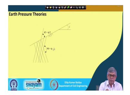
So, for that we can see, we can failure plane will be accordingly, so this is the one, so, with this with sorry. With respect to these, with respect to this is with respect to this will be 45 degree plus phi by 2 or 45 degree minus phi by 2 so that is the shown here.
