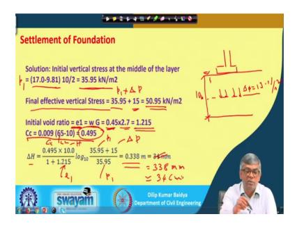
It is shown here you can see that, 1 second I will draw the problem and suppose clay layer is 10 meter and delta p equal to 15 kilo Newton per meter square. You can see that initial vertical stress at the middle of the clay layer so; that means, I have this is nothing, but p 1.
