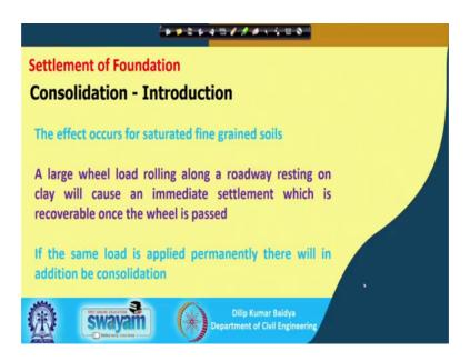
And this is the what is actually this is the effect happened to saturated fine grained soils and for example, elastic settlement and consolidation settlement if there is a large wheel load rolling along a roadway. And then we will see that the soil will immediately, the wheel will depress because of elastic settlement and when the wheel moves away from that point and then it will be mounts by the recover it actually the no permanent settlement.
