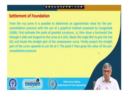
So, this is the procedure also written what I have mention, all are written here you have to draw a line on a from horizontal line from the point of maximum curvature then draw tangent. Then divide the angle then tangent from the state portion of the curve produced backward to intersect A D and find out locate the intersecting point F, from F you actually produce downward on the x axis and then read the x axis.
