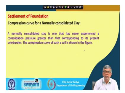
And then a normally consolidated clay is one that there is a in the there are in the field when you calculate consolidation there are two type of consolidation is there. One is normally consolidated, another is over consolidated; normally consolidated soil means what? The soil which has not been subjected to a higher pressure then the present overburden pressure.
