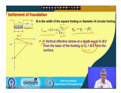
Similarly, he has given for a another type of footing that is which is applicable for square and circular square or circular footing and this is the diagram. You can see here this value is missing this will be 0.1 and you can see the diagram is almost similar only the value is changing you can see there actually at B depth from the base it was becoming Ie max.
