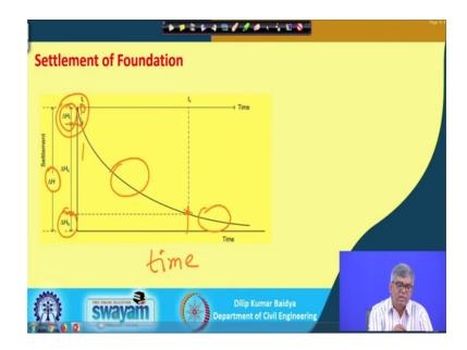
And you can see here that that is another point I want to highlight here that as I have told that there are three components; delta i delta c and delta s and if i plot this total consolidation total settlement over time settlement over time then you get a plot like this is time axis this is time.
