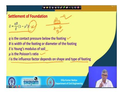
So, I will go to the next slide and. So, that you can see here that expression delta equal to qB E by 1 minus mu square I and q is the contact pressure below the footing; that means, if the footing is here. So, so through this footing what is the pressure? That is q and B is the width of the footing. If it is a rectangular then it is a smaller dimension if they strip
