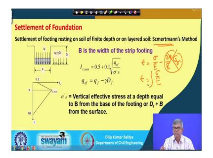
So, this is actually your plane actually the footing is resting on homogeneous elastic half space what is the meaning of it? That means, your footing is here and suppose and this one up to a great depth the homogeneous same soil is there and in that case that; that means, we have integrated 0 to infinity.
