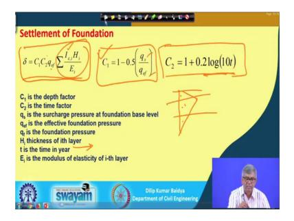
This is actually final expression of settlement equal to delta equal to C 1 into C 2 into multiplied by q effective sigma I Ei Hi divided by Ei and what is IEi?
