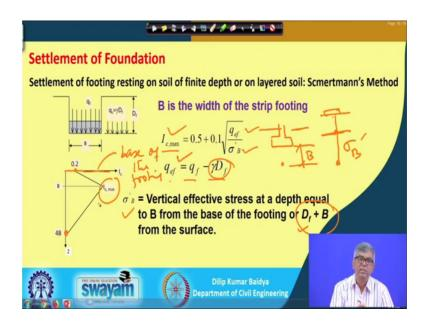
That this is actually this line actually it is just base of the footing base of the footing from here he has given a diagram the at the base of the footing value is 0.2 and at a depth of B that is instrument factor that is the Ie max I epsilon max and at 4 B depth that the epsilon that strain because of the load at this load applied at this surface at 4 B depth suppose strain is 0.
