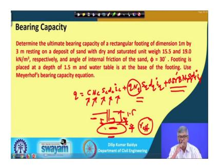
The problem is like this determine the ultimate bearing capacity of a rectangular footing of dimension 1 meter by 3 meter resting on a deposit of sand with dry and saturated unit weigh 15.5 and 19 kilo Newton per meter cube, that dry unit weight is 15 and saturated unit weight is 19.
