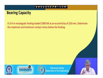
So, this is a A 2 by 3 meter rectangular footing loaded with 200 kilo Newton at an eccentricity of 250 millimeter and determine the maximum minimum contact stress below the footing. So, this is the problem we can see.
