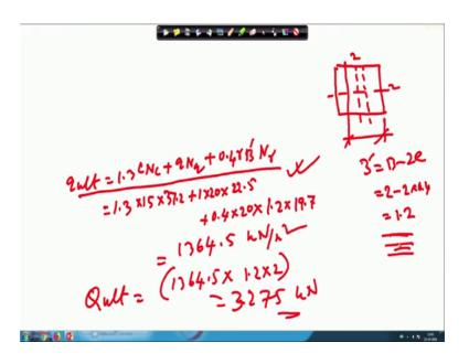
So, that means the footing is suppose this is 2 meter and this is 2 meter and eccentricity is 40 meter. So, what is the effective width actually that has to be you know B dash will be B minus twice e so; that means, B was 2 minus 2 multiplied by 0.4; that means, 1.2 meter. So, B dash is 1.2 meter and so in that case your q ultimate to be used as I have mentioned Terzaghi's theory is to be used and the square footing. So, 1.3 c cN c plus q N q plus q N q plus 0.4 gamma B dash N gamma.
