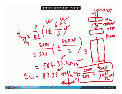
Footing is something, but low degree is applied here this eccentricity is 0.25 and this can be visualized as a concentrated load and there is a moment. So, moment become 2000 multiplied by 0.25 become 200 and this is two thousand p is p m equal to 500 p equal to 2000. And your footing dimension is this is 1 meter and this is this is 3 meter, 2 by 3 meter actually this is 2 meter and this is 3 meter.
