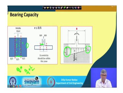
And, you can see now whatever I have shown actually we can see that you can see footing width can be divided by three parts B by 3, B by 3 B by at this is the center and exactly B by 6; B by 6 this is; that means, half of this. So, that is called one third rule, so, that means, the footing eccentric can be maximum can be this much or this much. So, that means, so, from here; that means, eccentricity maximum eccentricity can be B by 6, so, that means, B by 3 multiplied by half.
