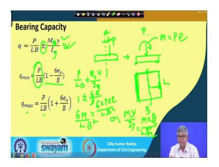
Now, you can see here as I have shown there if this is the footing and this is the centroid load is applied here and this can be considered as a loading and one moment and suppose your this is L and this is suppose B.
