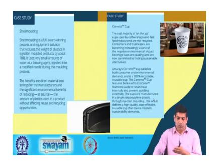
Then corretto cup which is another steam molding UK award winning process, they are doing some injection mould products by about reduces the weight by 10 percent. It uses a small amount of water as a blowing agent injected into the modified nozzle.
