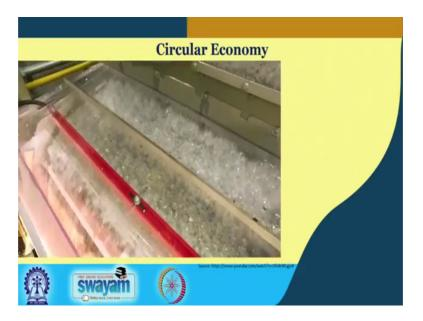
The our pet flakes which have come from the pet drinks bottles and other containers recycled around New Zealand. Now replace the majority of virgin or nearly pet in fact, state of the art high tech pet extrusion line in this process every roll of our pet foam is made in 3 layers.
