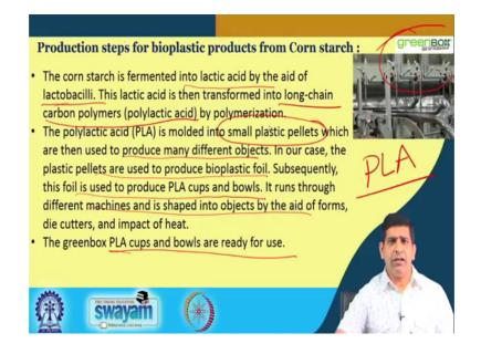
So, there are these are the production steps for bioplastic products from the corn starch the corn starch is fermented into lactic acid. So, if you can look at here they are forming lactic acid and by the aid of lactobacilli. So, in this lactic acid then transformed into a long chain carbon polymers which is called polylactic acid. In the short form you hear a lot PLA. So, PLA based plastic and that is the polyactic acid based plastic and this is molded into human day polymerization.
