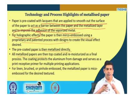
So, that is another area. So, in terms of these metallised paper what they are, this is paper is pre coated in with liquors, that are applied on is to smooth out the surface of the paper to act as a barrier between the paper and the metallised layer and to improve adhesion of the vaporized metal. Then you have a holographic effect, the paper is then micro embossed using a proprietary patent process create the visual effect desired.
