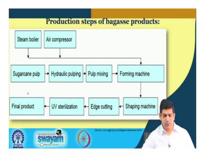
So, what how they are made it is from a steam boiler air compressor you will have a sugarcane pulp and that goes to hydraulic pulping, pulp mixing, forming machine, shaping machine, edge cutting, UV sterilization then you have the final product which is used for making those single use containers.
