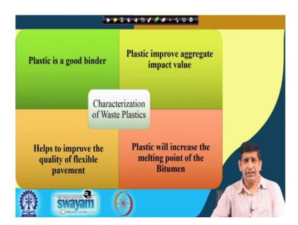
So, that is a its a why it works because, plastic is a good binder. Its a helps in binding those aggregates together, it improves aggregates impact value, it increases the melting
