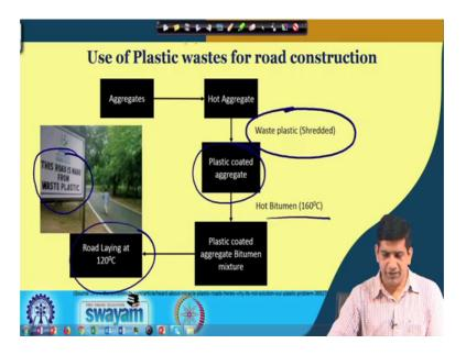
So, there are we go for plastic waste in the road construction. Any road construction you start with aggregates you will have hot aggregate and then you add plastic waste right there. We place plastic waste is added waste plastics ready they added to it that it gets plastic coated aggregate, this plastic coated aggregate with the hot bitumen. So, it gets
