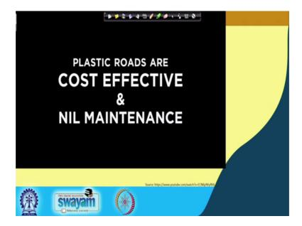
As you saw that the whole process in which the plastic waste was laid again it was essentially the similar process of what we do for our road construction, but again we are adding this plastic. We are adding plastic as explained in the previous slide as a first the plastic is shredded and then its added to the bitumen and mix with the aggregate first with the aggregate and then we add bitumen to it.
