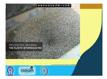
Fixed proportions of shredded plastic is added to the aggregate on a conveyor belt in a hot mix plant. It is then sent to the mixer where the shredded plastic melts and forms a layer on the aggregate. This process happens at temperatures between 170 to 180 degree centigrade. The plastic coated aggregate is then subjected to bitumen, plastic being a good binding material holds the bitumen together.
