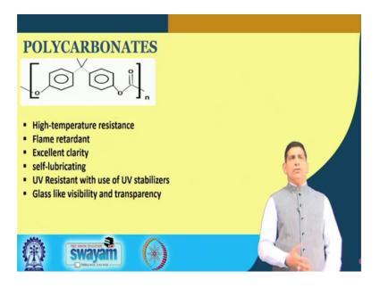
So, this is one example polycarbonate – high-temperature resistance, flame retardant, excellent clarity, UV resistance and the glass like material.
