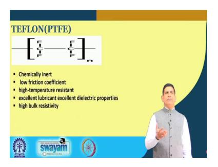
Teflon another chemically inert; Teflon, we use Teflon coated material excellent lubricant, excellent dielectric properties, high bulk resistivity.
