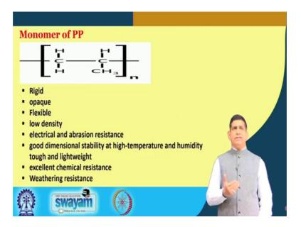
It is rigid; it is opaque; it is a flexible, low density; it is electrical and abrasion resistance, good dimensional stability, excellent chemical resistance, weathering resistance so that is
