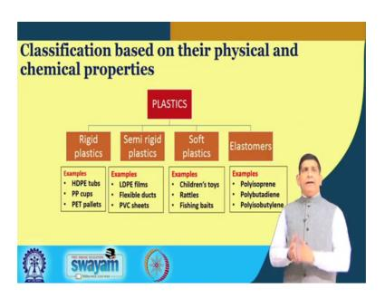
And then if you look at from physical and chemical properties, there are rigid plastic, which is very practice strongly HDPE tubs, polypropylene cups, PET pallets. They are very rigid. They will with and then you have semi-rigid plastic, which is LDPE films, flexible ducts, where you can have that is can move around a little bit, PVC sheets. So, these are semi-rigid.
