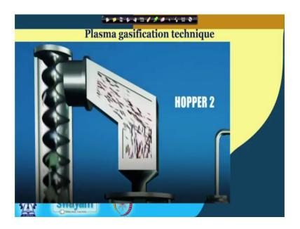
The second hopper connected to the gasifier supplies feed intermittently to the gasifier, but the feed read can be suitably adjusted by means of a control knob.
