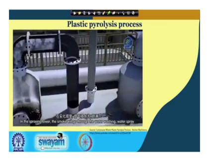
So, all these different steps is explained in great detail, then it is spraying tower, this small will go through the water washing and water spray did remove the air pollutants.
