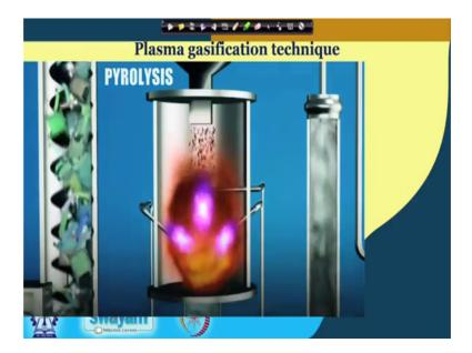
Pyrolysis or reactor is the heart of system, consisting a cylindrical chamber with a tapering bottom half. A transformer supplies necessary voltage to the graphite and carbon electrodes fixed inside the gasifier.
