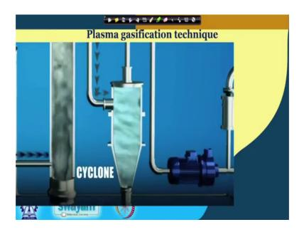
Cooled gas enters in a cyclone separator, which removes particulate impurities from the syngas through vortex separation. Rotational effects and gravity are used for separating impurities.
