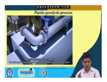
So, that whole process that we just explained and the hot smoke goes out of the reactor through inner pipe to the heat exchange system.
