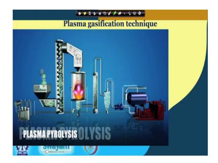
The technology plasma pyrolysis transforms high calorific thermal plastic wastes into a valuable synthetic gas, which can be applied well to gas turbines for power generation. It can also be used as a synthesis gas for hydrogen production.
