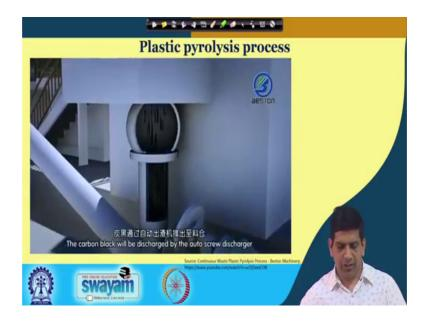
So, similarly in India it has to meet the Indian standard. The carbon black, which is collected is discharged through auto screw discharge. So, carbon black is collected as well, which can be used as adsorption material.
