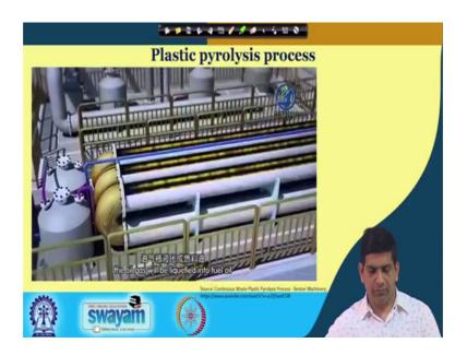
So, you have a then gas would be condensed in the horizontal tubular condenser. You have the condensation happening then they all gas will be liquefied into fuel oil.
