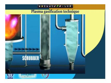
A slag removal system at the bottom of gasifier dreams, slag continuously in a water pot. High temperature in the gasifier generates syngas, which is passed through water scrubber for cleaning and quenching the hot gas. The con dude carrying the gas enters the scrubbing tower at the middle and water is sprayed from the top, the flow of gas is maintained by an i d fan which continuously sucks the gas.
