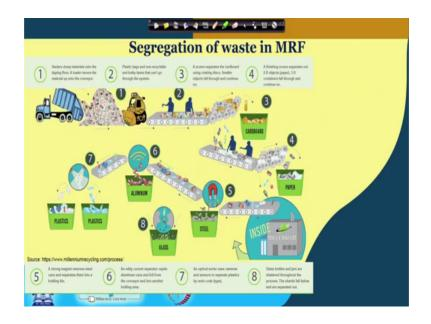
So, when we talk about this plastic waste. Plastic as you know in for most part, the plastic that we have to deal with is coming from the municipal solid waste. It is the m municipal solid waste the material recycling facility, which is also sometimes called as MRF, which is MRF as we actually stands for a Material Recycling Facility.
