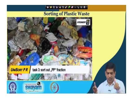
So, this is how things are getting sorted out then again it goes another round, which you will see here, it is trying to separate a P P fraction, which is the polypropylene fraction. So, that is coming out as well. So, it is so different fraction; we got P E T first out, we got H D P E out, now we are getting P P out.
