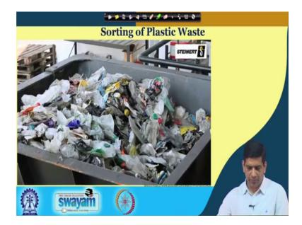
So, here as you can see the mixed plastic is getting loaded. So, this is your mixed plastic the container and then it goes into a conveyor belt and so, here overawed magnet, which
