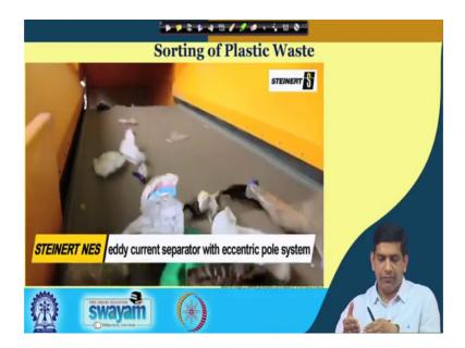
Now, after that you have eddy current separator; eddy current separated what it does? It tries, it removes aluminium cans.
