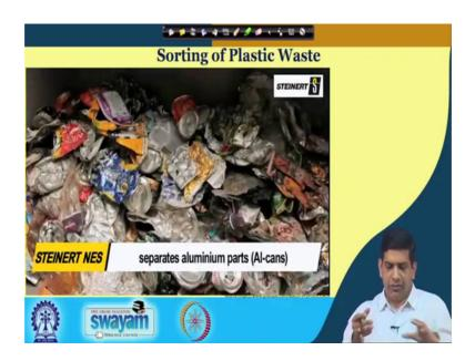
So, as you can see things gets blown away separates aluminium parts. So, anything with the aluminium gets blown away, in this eddy current separator which so aluminium is taken out. So, that can go as a aluminium waste. So, rest is now after removing iron, removing aluminium. So, in terms of the container system, you see the mostly now, its your plastic.
