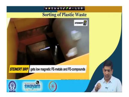
It gets low magnetic iron material and iron compounds, so, even that is removed out. So, you see those which traces of so many times, what happens? This packaging material has mixed shear stuff. So, that is that needs to be removed. So, though becomes contaminant.
