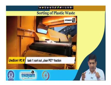
So, it is a hyperspectral sensor sorter. So, this sensor sorter what it does? As it is taking out clear P E T fraction, the first task it does; it's tries to remove this clear P E T. So, anything clear P E T bottle, it is removing that and then again it is on the conveyor belt and it will. So, these plants you see lots and lots of conveyor belts, things just moving around. Then you have another sensor sorter after removal of the P E T it will go for, I think H D P E, yes.
