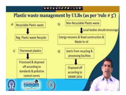
So, for ULB's they have to take recyclable plastic waste and non recyclable. Recyclable plastic waste which can go to registered plastic waste to recycle or again these things the rules have been in place for quite or more than 2 years like for almost 2 years now, but it still if to find a plastic waste registered recycler even in big cities you will not find that much. We don't have there are some for which many of them are not functional that much.
