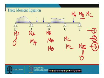
Now, we have the relation between M A, M B and M C. Now, we have relation between M A, M B, M A, M B and M C right. Now, M A, M B, M C are means we have a relation between three cons moments in three consecutive, three consecutive supports. If we are considering the compatibility conditions at B, then we have relation between M A, M B and M C, but if we compute the compatibility equation at A, then we have a relation between M D, M A, M A and M B that is for compatibility equation at A.
