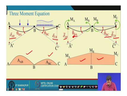
Now, suppose under the action of these external load, this is the deflection. And now by looking at the deflection pattern, you can easily make that the though there is a that that these a at the deform shape is continuous at B, but it is not differentiable at point B, the slope is not continuous at point B ok. Because the rotation at this point rotation of segment A B and rotation of segment BC, they are they could be different ok.
