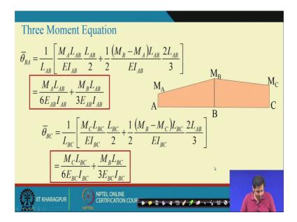
Then the theta B A bar means the angle at B A rotation at B A in segment rotation at B in segment B A can be obtained like this. And similarly rotation at B, in segment B C can also be obtained like this.
