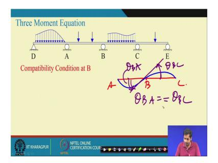
Now, this are the theta B and theta B C, now let us see what is the compatibility in this case you see. The compatibility conditions will be suppose if we a if we take any continuous beam, suppose it is a this is A B and this is C. And suppose deform shape in these structure deform shape is suppose something like this something like this ok.
