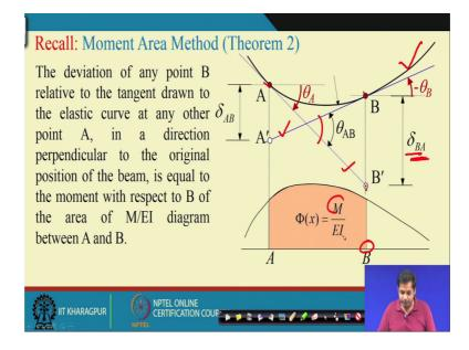
Now, we need to recall one important theory the moment area method, the moment area method there are two theorem of moment area method, theorem one says that how to compute the slope at a given point and then theorem two tells you how to calculate the deflection at a given point.
