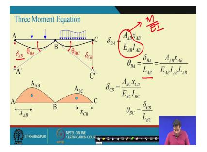
Now, then if you do that then, this is the suppose x AB, x CB are the centroid distance of centroid from A and C and, then delta B A is equal to am this is the movement M by E I diagram, this is the area of the moment and this is M I E I diagram M by M by E I diagram.
