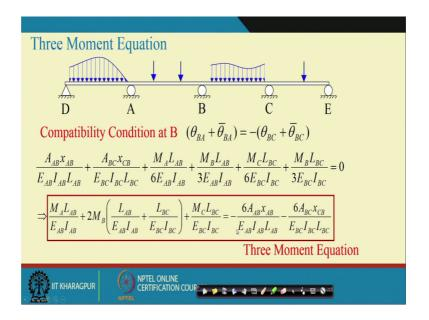
If we substitute the correspondent values then, we have these equation So, these is called three moment equation the reason is three this is called three moment equation, you see these equation actually relates moment M A and, then moment M C and, then moment and then moment M B. And other then this three moments M A, M B and M C all other parameters you look at this equation, all other parameters are known. So, only none known unknown in this equation M A, M B and MC.
