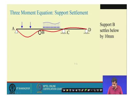
Now, another important addition in or in important part in three moment equation is the it supports settlements, you see suppose in a continuous beam, if any support settle any support settles means, if there is a displacement in support that could be because of anything, because of the construction problem, because of the of the sinking of the structure, because if the settlement of the soil, it could be anything. But it any case if
