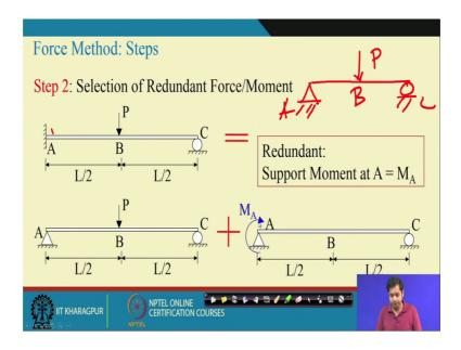
This structure is still determinate structure and not only that it is stable structure so we have removed the moment at the moment constraints at A so in this case the moment at A in A is taken as redundant forces.
