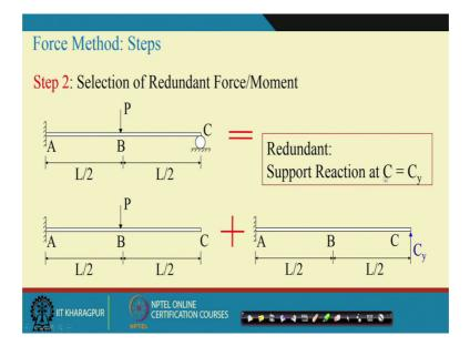
So, once it is done again go back to our original problem the this problem; so let us continue the analysis by taking C x as the redundant C y as the redundant. Now if I take C y as the redundant this are the basic indeterminate structure; now the next step in these
