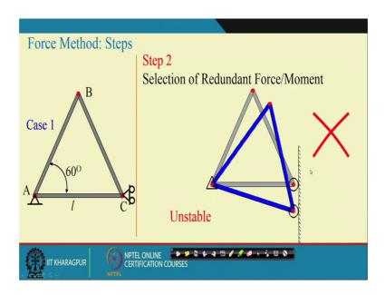
Case 1 is this one is the case 1 where  $C \ge C \ge y$  is the redundant forces; now if it is subjected to a  $C \ge x$  is a redundant forces; now you see if it is subjected to if it is subjected to some load some load P then this may deform like this you are this may this may collapse entire structure may collapse like this.
