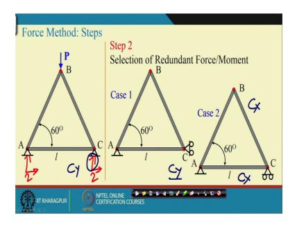
Take another structure another truss; which is again determine indeterminate structure if you can see here the number of reactions are 2, here also number of reactions are 2, so here it is 2, here it is 2; so total number of reactions are 4, but as a per as the number of reactions are concerned we can have 3 equations so it is redundant forces 1 static indeterminacy is 1 ok.
