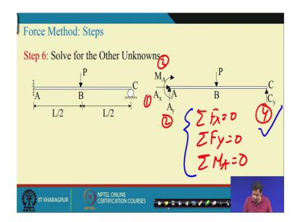
So, now once we know the reaction at point C the next step is to next step is this is now known; if you apply the free body diagram this is the free body diagram in this free body diagram initially before doing all this exercise initially we had four unknowns A x A y 1 2 3 and then 4, we had 4 unknown, 3 equations summation of F x summation of F y summation of F x is equal to 0.
