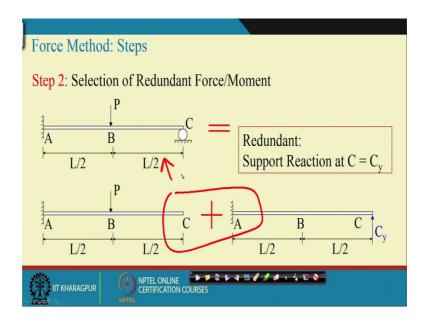
Now if you do that if you take this as a redundant force so F you do that this as a redundant force next step is we have to use it based on this redundant force we need to decompose the entire structure into basic indeterminate structure.
