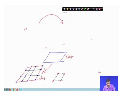
When we say that when we say that an element is for instance if we take this case in this case, your actual points actual in area was this, which is an continuous system having infinite number of points, thereby having infinite number of degrees of freedom.
