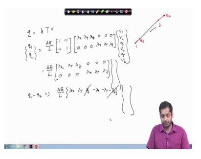
So, what we have is q is equal to q is equal to k, k into T into v right. Now, if we have this is the member in the cross at this point you your force is q, these points it is 1, this point is 2, here you have q 1, and here you have q 2, q 2. So, the forces in this member will be q 2 minus q 1. So, say let us let us calculate, what is q 1 and q 2, only thing is only thing is you have solved for the unknown displacement global displacement right.
