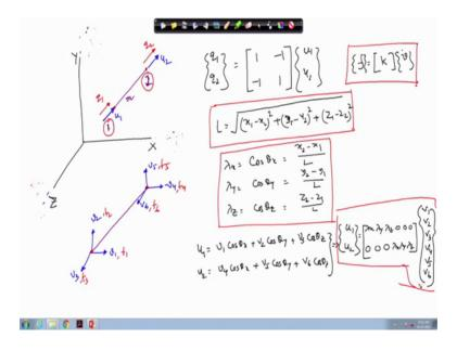
Suppose, let us fix our coordinate system, we have a coordinate system like this, we have a coordinate system this, this and this. Suppose this is X, this is this is this is Y and this is Z right. Now, we have a truss say this is a truss, this is the truss, this is a truss member, any truss member say m, truss member m. And this is ith point and this is jth point.
