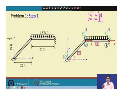
So, now here naturally the first impression is to discretize in this form because this is node 1, node 2, node 3 and there is a node 1 corresponding to 1, 2, 3, degrees of freedom node 2, 4, 5, 6 node 3, 7, 8, 9. So, among these 9 degrees of freedom 6 degree kinetic degrees of freedom are known to us because 1, 2, 3 we all know there is no rotations no horizontal and vertical displacement. So, 1, 2, 3 is known and similarly 7, 8, 9 is also know.
