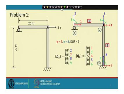
So, in the last class we have solved one example, this example is essentially a twomember plane frame. So, in this frame there is a horizontal load of 5 kilo pound and the one end is fixed and another in this ruler supported. So, we solve this frame by matrix method or specifically the stiffness method and this is our degrees of freedom.
