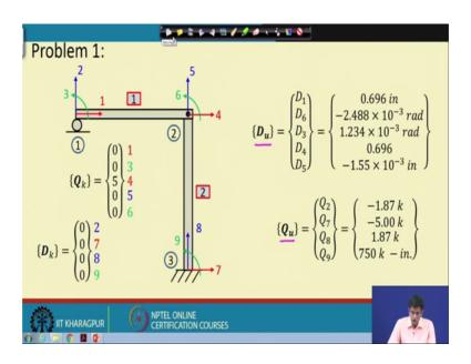
The solution is this we have solved in the last class. So, this is the D unknown; that means, the partitioning of after partitioning of the matrix you obtain this solution and then once we obtain D unknown. So, we obtain Q unknown by the second equation of the matrix equilibrium equation.
