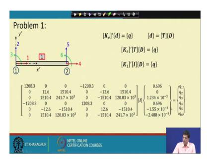
So, just by substituting this D 1 to D 6 that is that we have found out in the previous class if we substitute it here we get q 1, q 2, q 3 and qc, q 4 and q 6.
