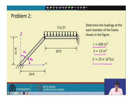
Now, let us do another problem which is an inclined member essentially this member is inclined along with an theta with x axis so, this theta can be found out. So, essentially what we need is theta x and theta y with the member that is inclined with the x axis. So, this is my global y axis so, this member both the ends of this member are fixed.
