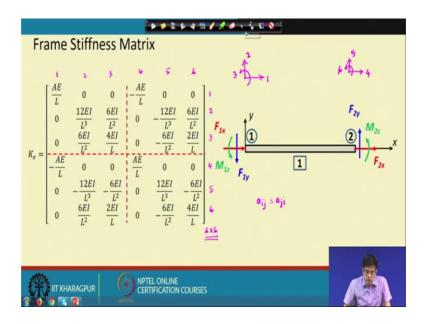
So, this is the frame stiffness matrix so, we know what are the frame stiffness matrix here. So, we know what are the degrees of freedom and essentially we find out 6 cross 6 stiffness matrix.
