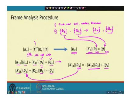
What is the frame analysis procedure? So, the frame analysis procedure in general is very similar to the stiffness analysis procedure where actually we have seen it for a truss, we have seen it for beam. For instance, if you have a structure if first you determine the degrees of freedom what are the degrees of freedom? Then actually you discretize or find
