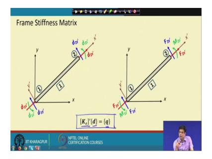
So, in a first let us understand in a local coordinate system or local the elemental coordinate system what is the equilibrium equation?
