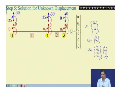
So, step 5 is solution for unknown displacement. Now, this is the displacement vector, all these displacements are known. Suppose, if you recall if we can write this, we can express u as; we can express u as; say u is equal to u unknown, and u known. And u unknown is equal to in this case, u 1 u 2; and u known in this case is u 3 u 4 u 5 u 6 which is  $0\ 0\ 0\ 0$  right. So, this is how we can write.
