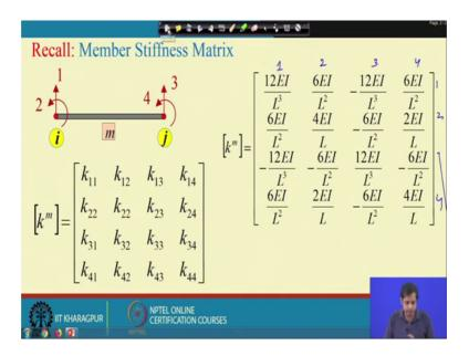
Now, just before that recall this we discussed in the last class. If we have a member, connecting connected between two point, two nodes i and j, and the degrees of freedom at i<u>t</u> node is 1, 2, and degrees of freedom that jth node is 3, 4, then this is the stiffness matrix for this member general stiffness matrix for this member.
