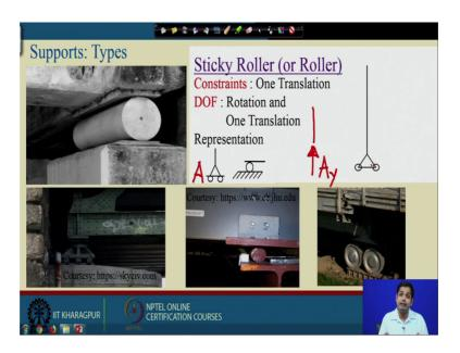
Now, next another support is another support is roller support. As you can see here the motion in this direction is constrained, but the displacement if the moment in this direction is a moment in this direction is allowed. So, it has rotation degrees of freedoms are rotation and one translation. So, this can rotate about this and this can translate about this.
