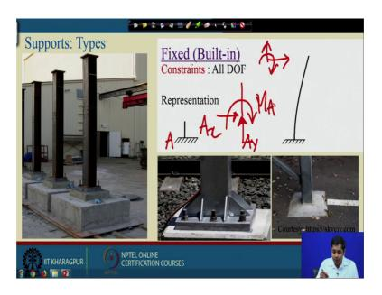
For instance we have fixed support. Fixed support means this is the this is the way we represent fixed support you are so, you all are familiar with all this these are some examples of fixed support. So, what are the diff in fixed support the degrees are constraint are all degrees of freedoms are constrained.
