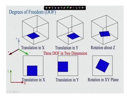
Now, if we take a problem in 2 D, then in two dimensions we have three degrees of freedom, this axis is where the object lies in plane. So, you have you can have two rotate, two translations and one rotation two translation and one rotation. So, these are the three degrees of freedom we have of an object in two dimensions ok.
