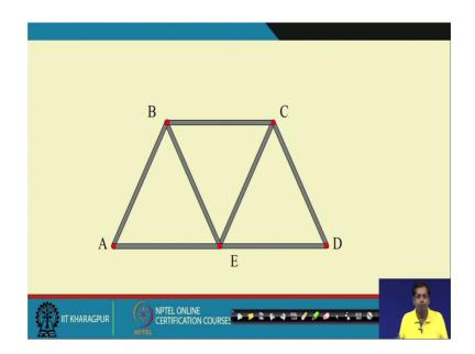
So, let us take a truss problem. Now, if we the first step is we remove the take only this truss, remove the loads, remove the boundary conditions, how to use the load and the boundary conditions we will see in the subsequent lectures. Now, this is the structure we have
