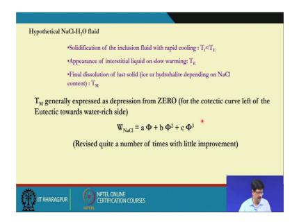
So, in a hypothetical NaCl is to fluid; the solidification of the inclusion fluid will be rapid with rapid cooling the freeze temperature at which it will I; it will completely frozen which you can represent is T f will be much less than that of T E corresponding to eutectic temperature in the binary.
