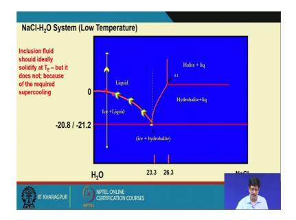
Ok. So, now, we move on to the response of aqueous biphase inclusion to heating freezing experiment and will start with freezing first. This is diagram which you have already discussed is a binary water NaCl diagram and this is only up to limited compositional range.
