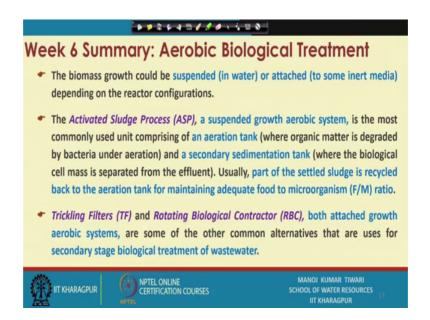
The biomass growth could be suspended or attached; so, the suspended growth are where the microorganisms remains in suspension within the water; whereas, in attached growth system they grow on the surface of some media. So, there is some inert media it is provided and on the surface of these media the biomass grows slowly and as a result form the bio film ok.
