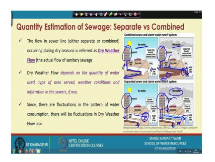
We can multiply them and get the estimate of the quantity of the sewage. Now, the sewerage system typically are of 2 types, the separate system separate sewer and a storm water runoff system and the combined sewer and storm water runoff system.
